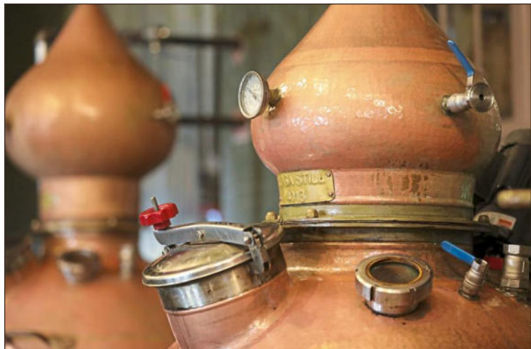
A copper still is used to heat and separate the components of rum made at Tim Russell’s Maggie’s Farm Rum distillery in the Strip District.
